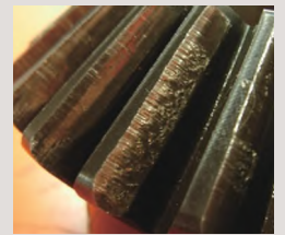
Example of wear due to insufficient surface durability
